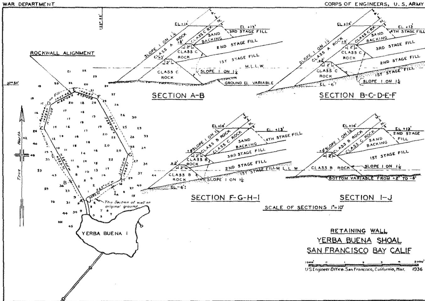
Fig. 3.36: Configurations of Perimeter Rock Dikes; Treasure Island [U.S. Army Corps of Engineers, 1937]
