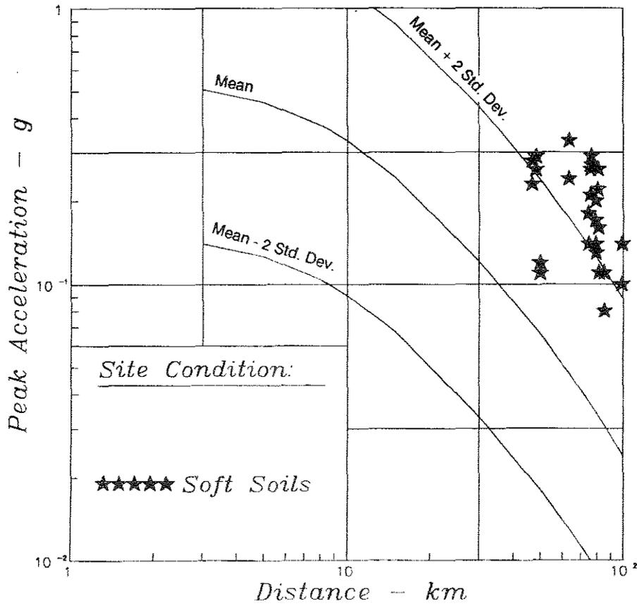
Fig. 4.6: Recorded Peak Horizontal Ground Surface Accelerations on Soft Bayshore Sites, and Attenuation Relationship Proposed by Joyner and Boore (1988)
