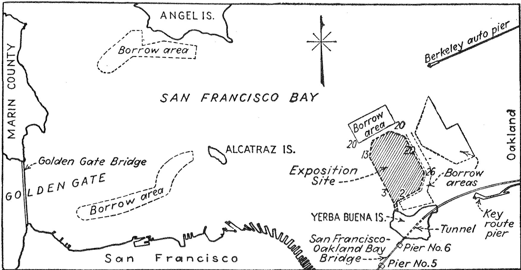
Fig. 3.35: Map Showing the Location of Treasure Island ("Exposition Site"), Yerba Buena Island, and Dredge Borrow Areas from Which Fill was Obtained [U.S. Army Corps of Engineers, 1937]
