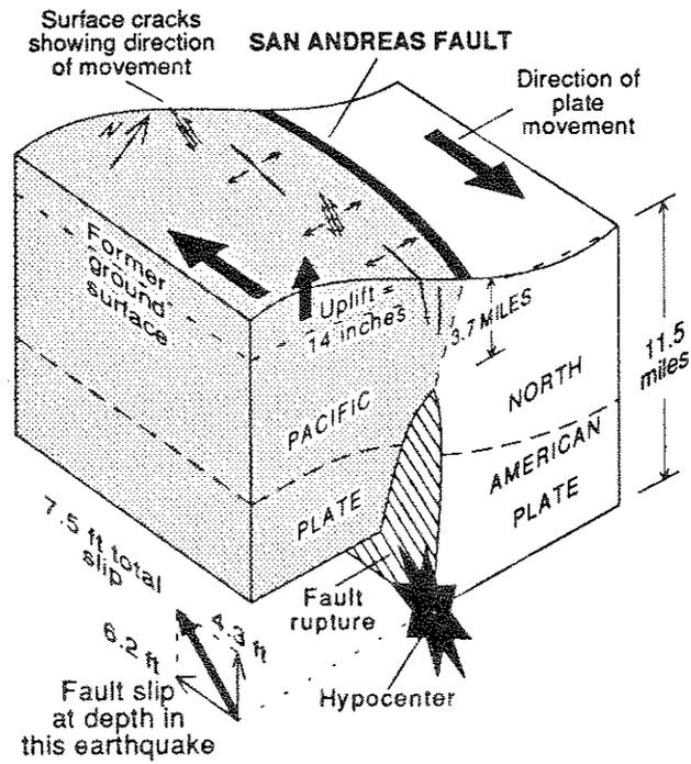
Fig. 2.2: Schematic Illustration of Estimated Fault Movements;
