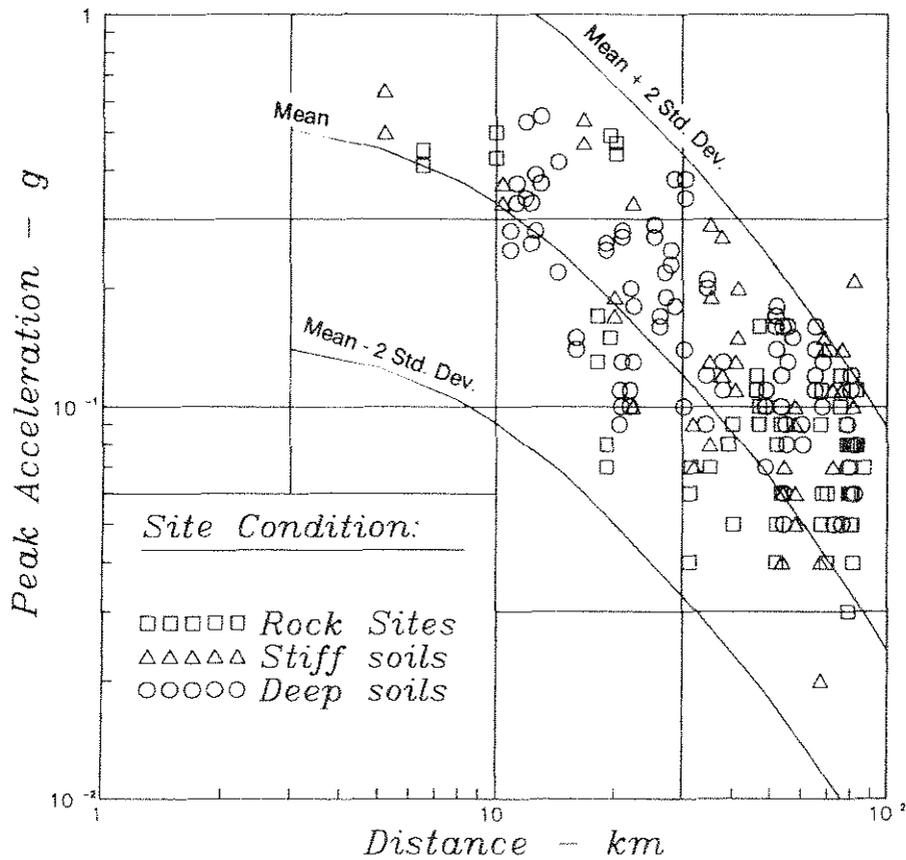
Fig. 4.5: Recorded Peak Horizontal Ground Surface Accelerations for All Site Conditions Except "Soft Soils", and Attenuation Relationship Proposed by Joyner and Boore (1988)
