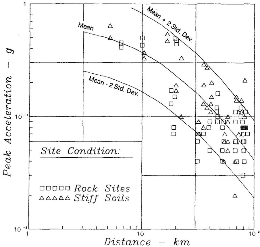
Fig. 4.4: Recorded Peak Horizontal Ground Surface Accelerations on Rock and Stiff Soil Sites, and Attenuation Relationship Proposed by Idriss (1985)
