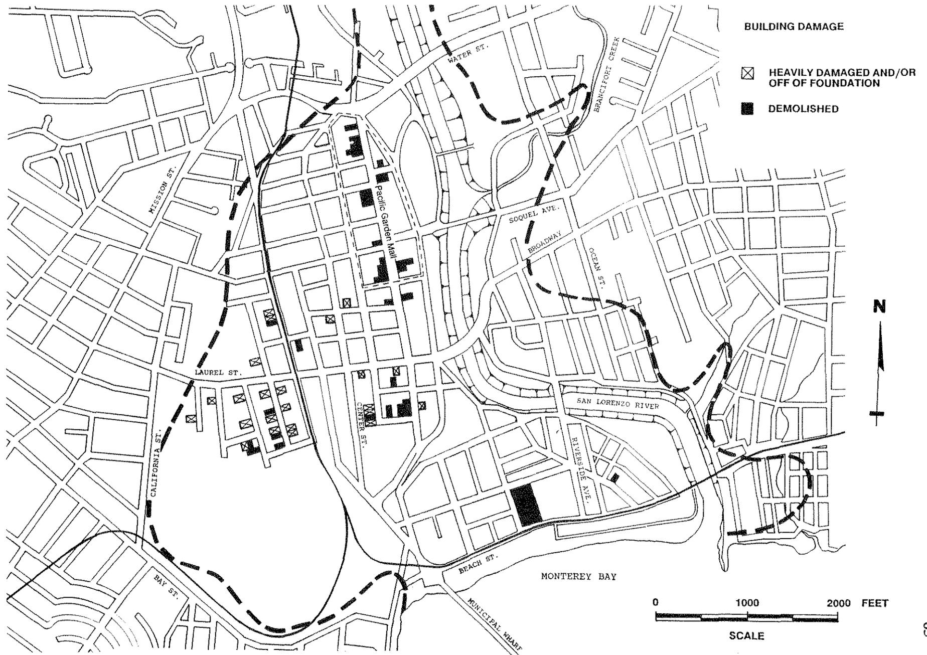
Fig. 3.78: Map of Central Santa Cruz Showing Locations of Demolished and Heavily Damaged Structures
