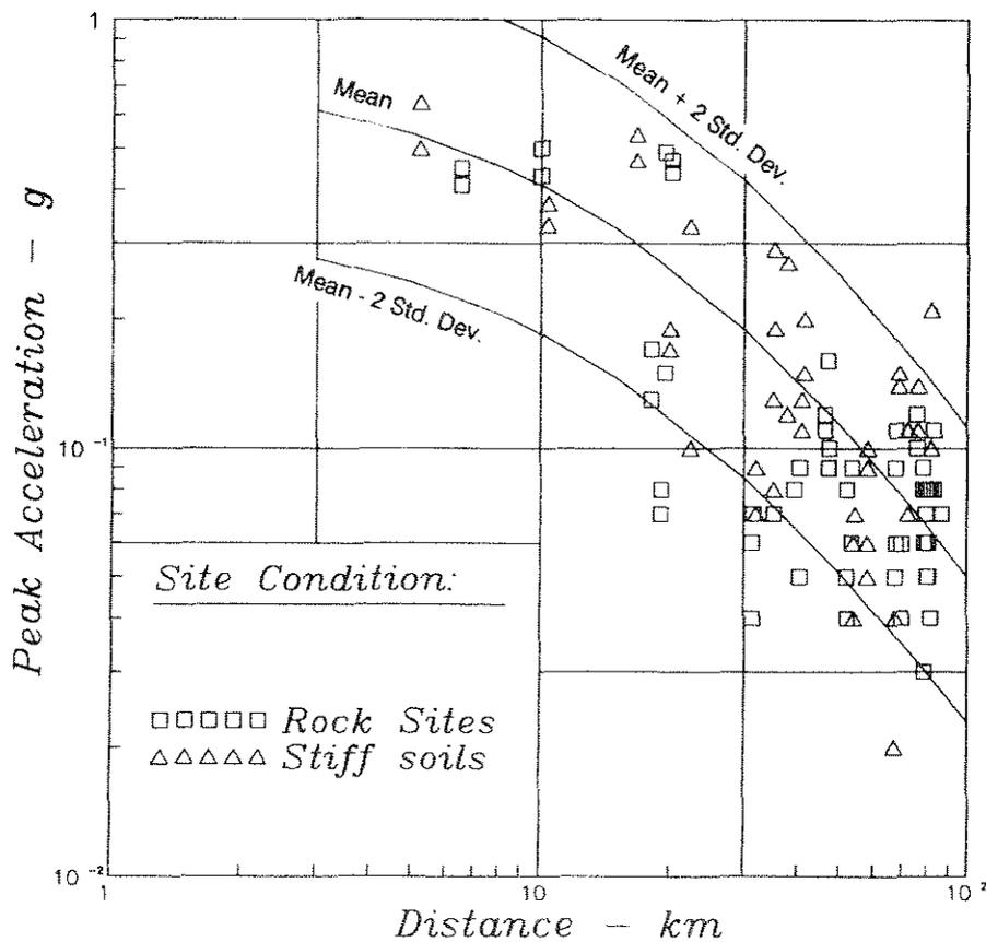
Fig. 4.3: Recorded Peak Horizontal Ground Surface Accelerations on Rock and Stiff Soil Sites, and Attenuation Relationship Proposed by Seed and Idriss (1982)
