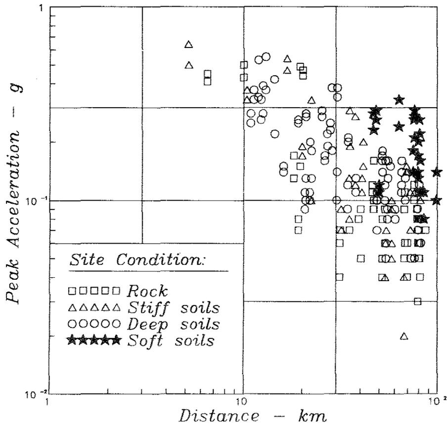
Fig. 4.2: Recorded Peak Horizontal Ground Surface Accelerations vs. Distance from the Fault Rupture Surface
