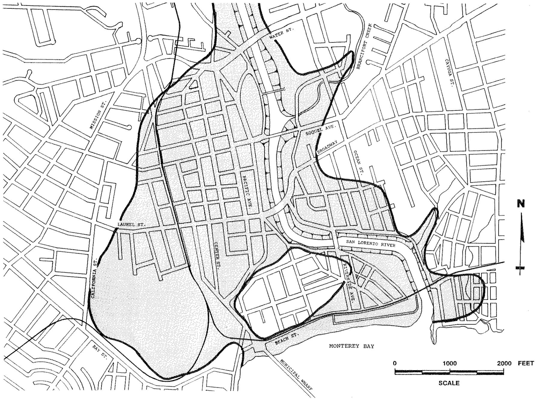
Fig. 3.73: Map of Central Santa Cruz Showing the Zone of Highest Risk of Soil Liquefaction
