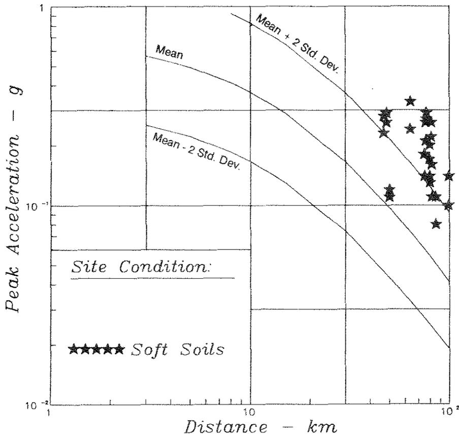
Fig. 4.7: Recorded Peak Horizontal Ground Surface Accelerations on Soft Bayshore Sites, and Attenuation Relationship Proposed by Idriss (1985)
