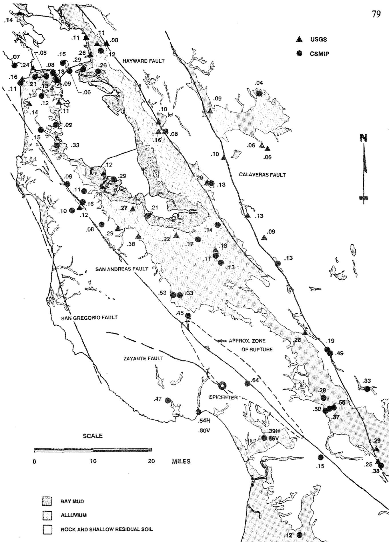
Fig. 4.1: Overview of Regional Geology and Recorded Peak Horizontal Ground Surface Accelerations During the Loma Prieta Earthquake of October 17, 1989
