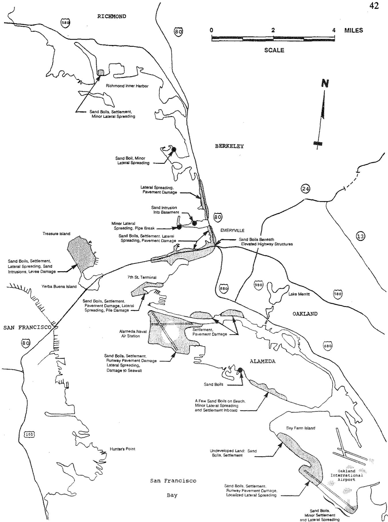
Fig. 3.45: Map of the East San Francisco Bay Shore Region Showing Sites Which Experienced Liquefaction During the Loma Prieta Earthquake of October 17, 1989
