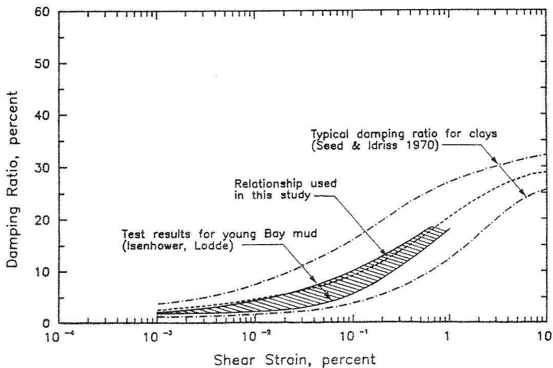
Fig. 4.23: Variation of Dynamic Shear Modulus and Damping Ratio with Shear Strain for Young San Francisco Bay Mud (Seed and Sun, 1989)
